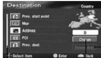
This bar indicates that there is a continuation of the list. Tilt the joystick to scroll the list.
