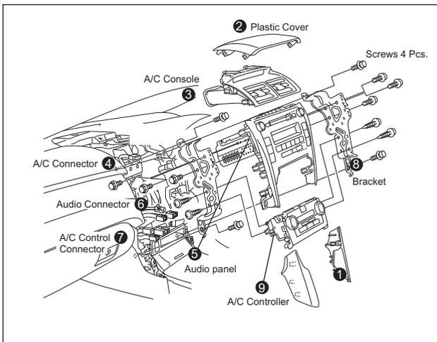
1. Remove part no. ① by removing all clips off.
