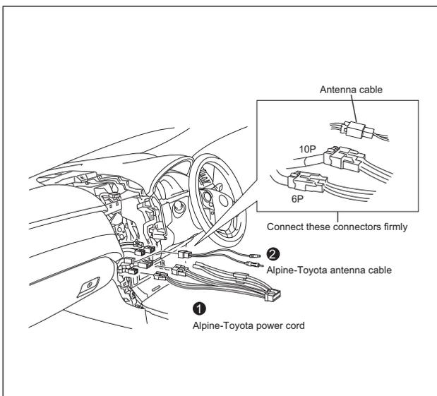
1. Connect the Alpine-Toyota power cord ① into the car connectors both 10P and 6P.
