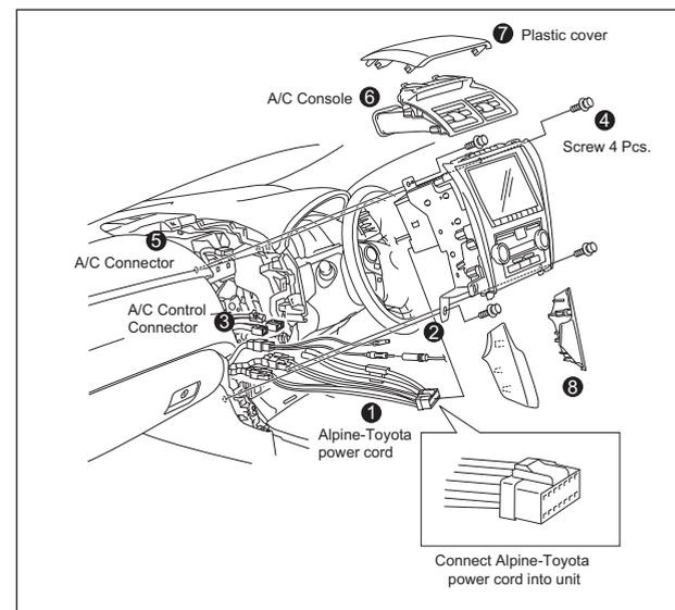
1. Connect the Alpine-Toyota connector ① and the Alpine-toyota antenna cable ② into the head unit tightly until you hear "Click".
