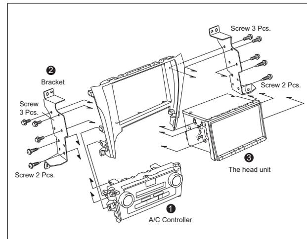
1. Connect A/C controller ① with audio panel by pressing all clips tightly.
