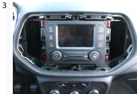
3 Remove and save the 4 screws circled in Red. Disconnect all cables and remove the OEM Radio from the radio tunnel.
