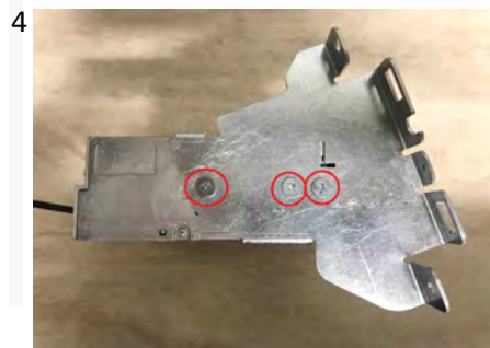
4 Fix the brackets to the Radio by tightening the 3 screws per side supplied in the kit.
