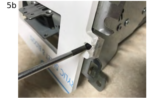
5 Fix the fascia plate to the brackets using the 2 black screws and the 2 spacers as shown in the picture 5a.
