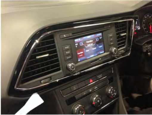
1. Remove the plastic trim from around the head unit and air vents using a plastic removal tool.
