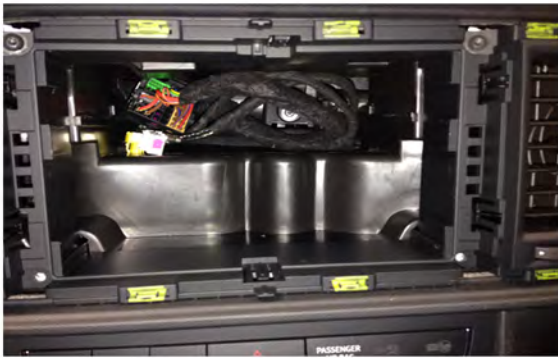
3. Image of the head unit removed and all wiring connectors disconnected.
